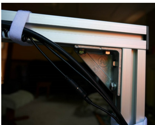
Figure 3 a top bar bracket - also note the use of the velcro wrap to tidy cables
