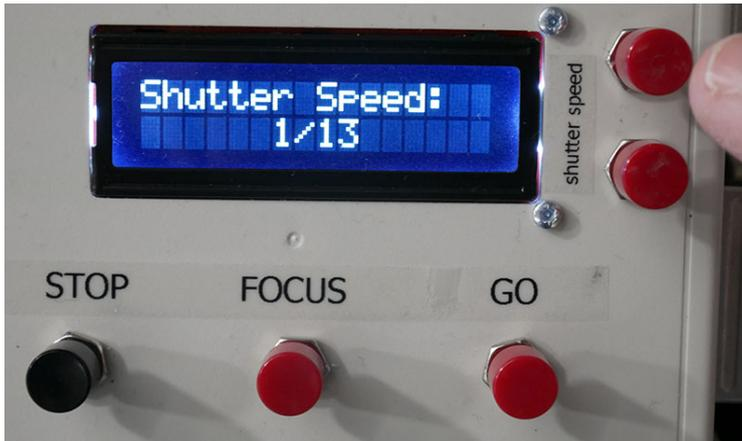
You must set the shutter speed using the Up/Down buttons to the side of the screen. This cycles through all possible shutter times and is used to calculate how long the lights are on. If it is too long (eg 1/2s instead of 1/4s) it will still work but take longer to capture.
