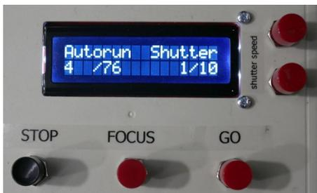
Press the GO button and the full capture process will run, showing which LED it is currently using.
