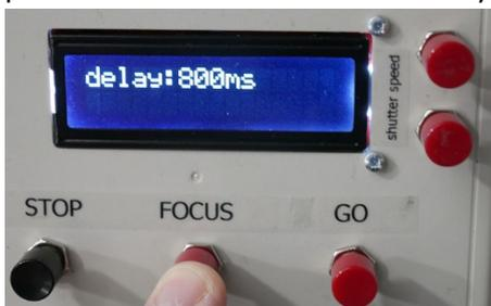
The best speed depends on the camera and how fast the memory card is. If this delay is too short the camera may stop capturing as its buffer overflows. You can then increase the value by say 300ms for a reasonably safe value. Capturing RAW will require a longer delay if you have a slow card. If your sequence includes black images that is a sign that the timing went wrong.
