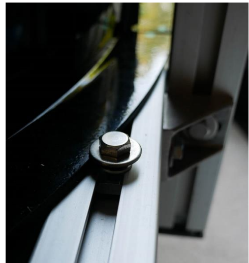
Figure 3 dome retaining bolts - there are four of these which help to keep the dome in the same place. Hand tighten only.
