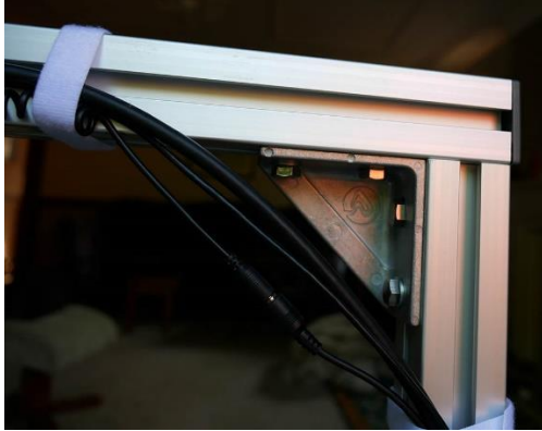
Figure 2 a top bar bracket - also note the use of the velcro wrap to tidy cables
