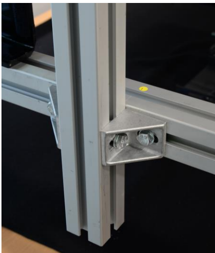
Figure 1 The vertical bars have some adjustment so you need to tighten a bolt when they are vertical. The third bracket underneath can be attached last when the top bar is levelled
